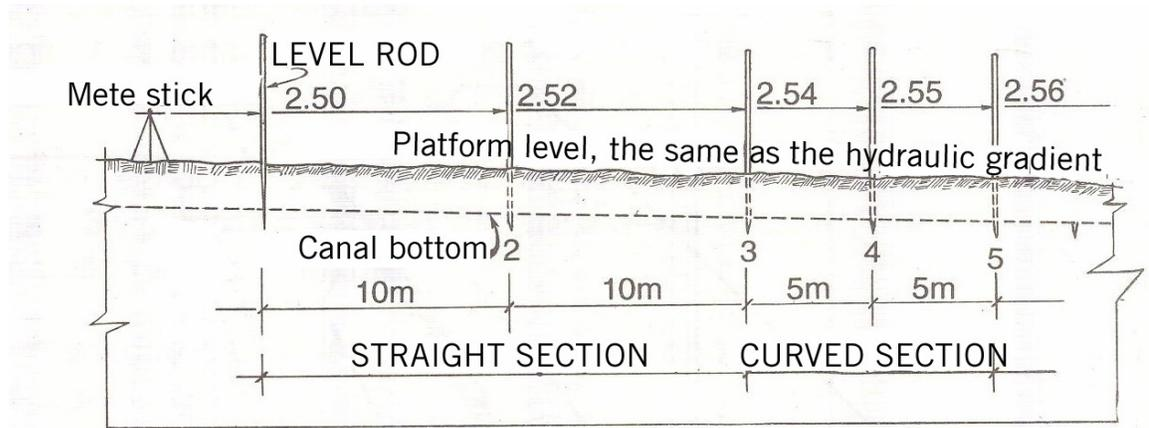
Slope: 2/1000 (two per thousand), which means that every 10 m horizontally there is a difference in elevation of 2 cm and every 5m horizontally there is a difference in elevation of 1 cm.
